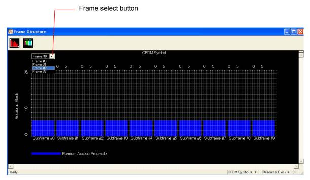
Figure 3.1.7.1-2 Random Access Preamble Setting Screen
