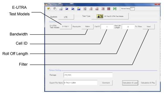
Figure 4.3.2.1-1 BS Test/E-UTRA Test Models Common Setting Screen
