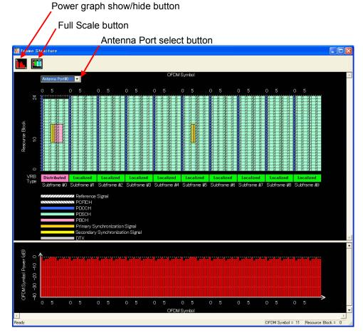
Figure 3.1.7-1 Frame Structure Screen and Power Graph
