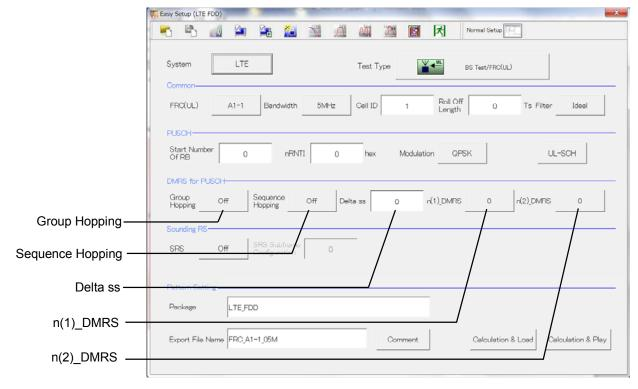
Figure 4.3.3.3-1 DMRS for PUSCH Parameter Setting Section
