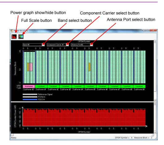
Figure 3.1.7-2 Frame Structure Screen and Power Graph (LTE-Advanced)
