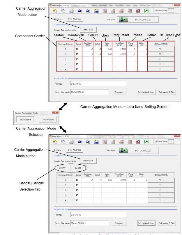
Carrier Aggregation Mode = Inter-band Setting Screen
