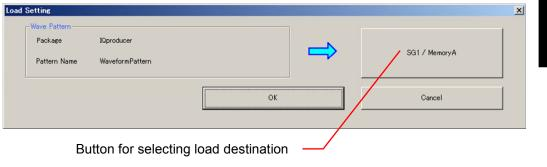
Figure 3.1.10-1 Load Setting Screen
